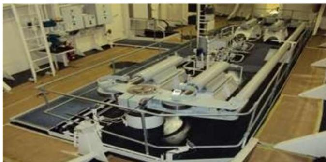
Gambar 2.4 Four ram hidraulik steering gear
