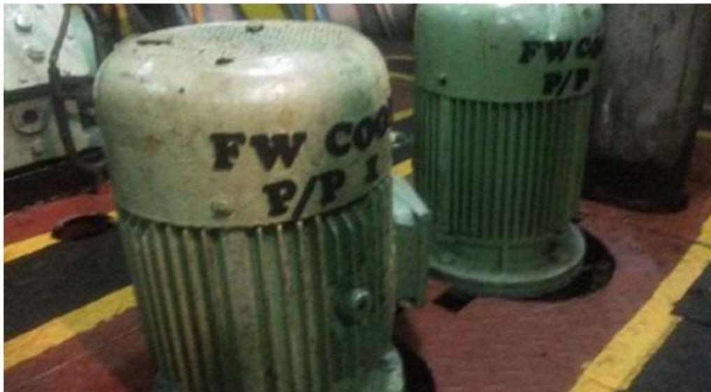
Gambar 2. 3 Pompa Sirkulasi Air Tawar
