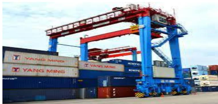
Gambar 2.2 *Rubber Tyred Gantry Crane (RTGC)*
