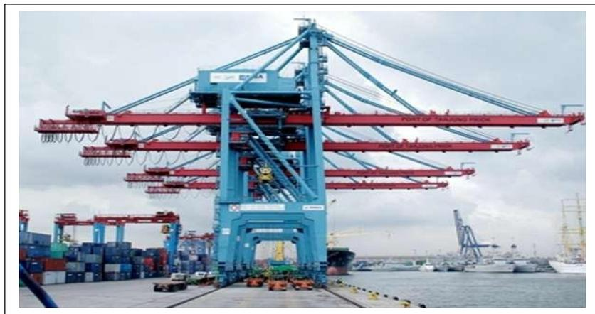
Gambar 2.7 *Quay Container Crane*
