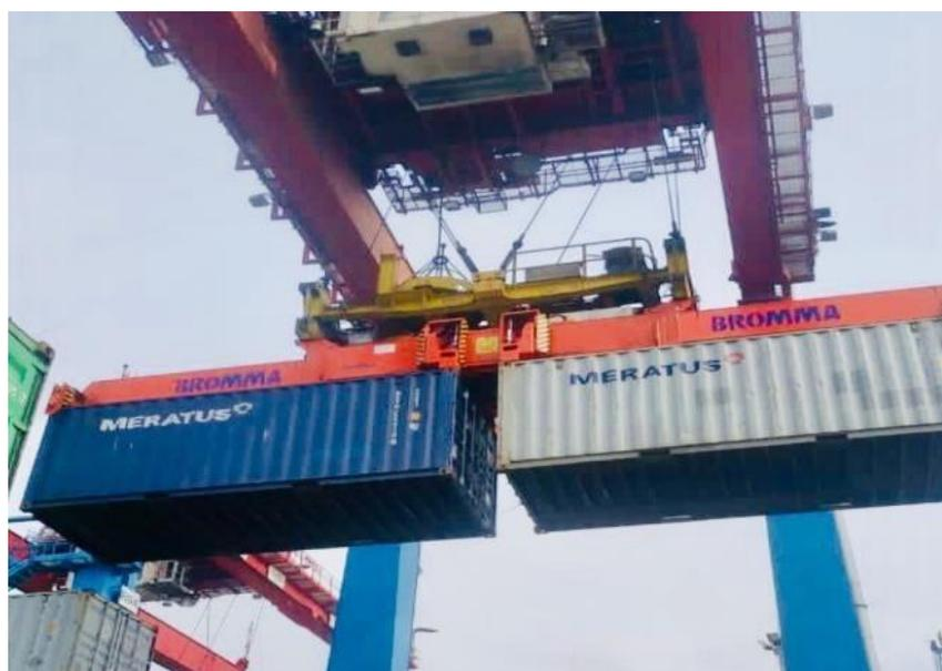
Gambar 2.11 *Spreader Twin Lift mode*
