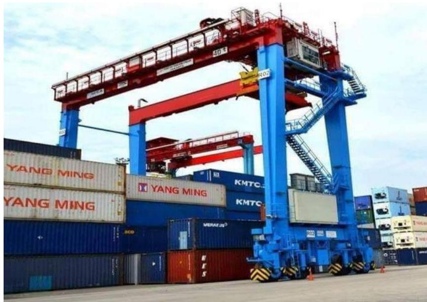
Gambar 2.9 *Rubber Tyred Gantry Crane ZMPC*.
