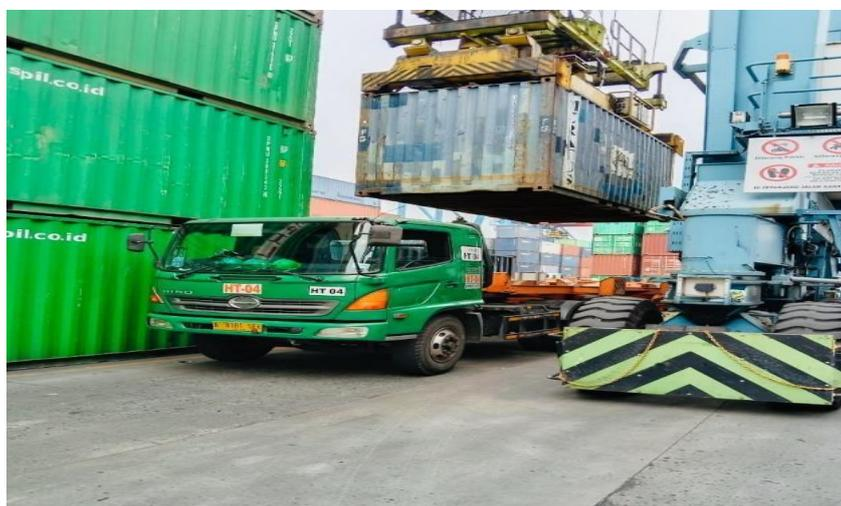
Gambar 2.10 *Spreader Single Lift*
