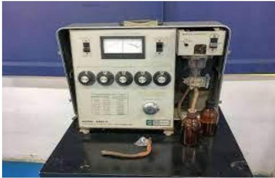
Gambar 2.5 Salinometer
