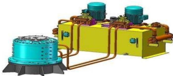
Gambar 2.7 Rotary vane steering gear
