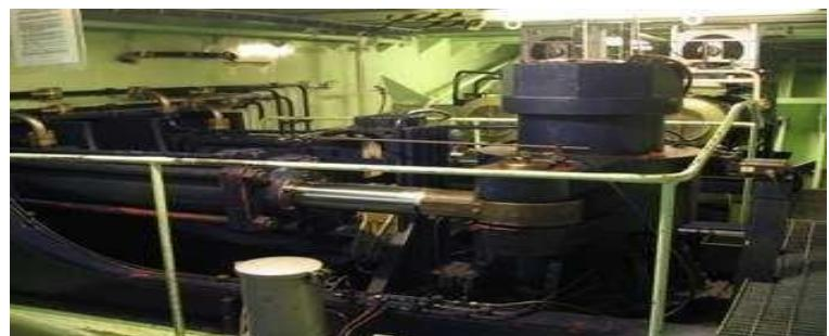
Gambar 2.2 electric steering gear
