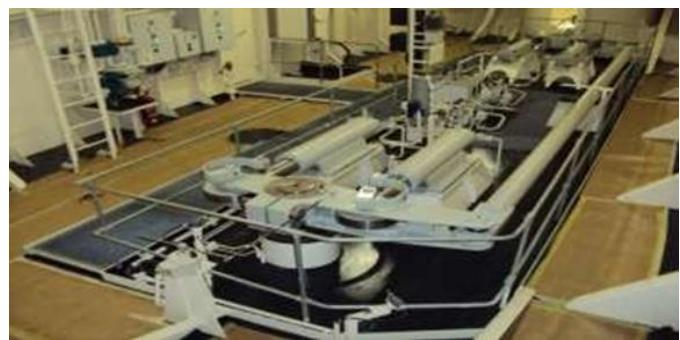
Gambar 2.4 Four ram hidraulik steering gear
