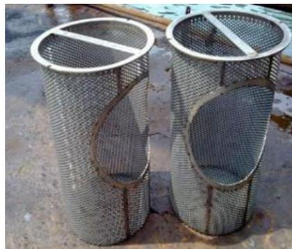
Gambar 2.4. Filter pompa *ballast*
