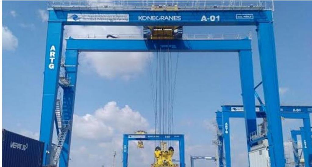
Gambar 7 *Automatic Rubber Tyred Gantry*
